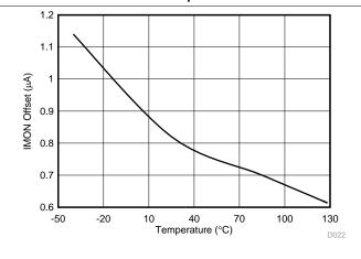
Figure 22. IMON Offset vs Temperature
