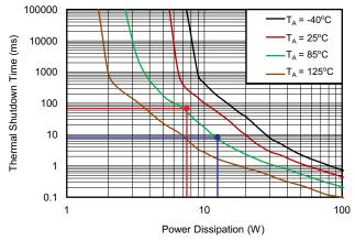
Taken on 2-Layer board, 2oz.(0.08-mm thick) with GND plane area: 14 cm<sup>2</sup> (Top) and 20 cm<sup>2</sup> (Bottom)
