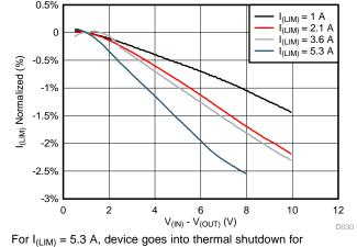
For  $I_{(LIM)} = 5.3$  A, device goes into thermal shutdown for  $[V_{(IN)} - V_{(OUT)}] > 8$  V
