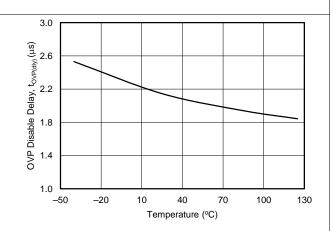
Figure 9. Enable Turnoff Delay vs Temperature
