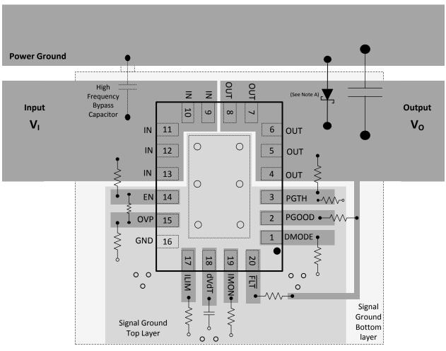
A. Optional: Needed only to suppress the transients caused by inductive load switching.
