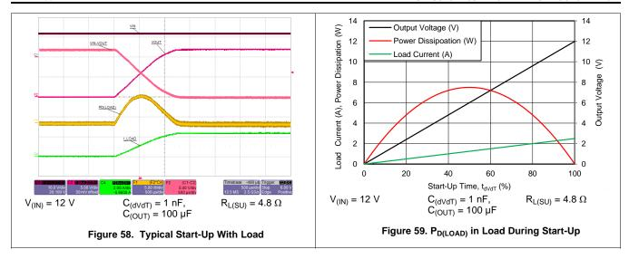
Solving Equation 20 the average power loss in the device due to load is given by Equation 21.
