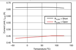
Figure 20. Current Limit for R<sub>(ILIM)</sub> = Open and Short vs Temperature
