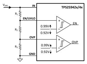
Figure 50. UVLO and OVP Thresholds Set By R<sub>1</sub>, R<sub>2</sub> and R<sub>3</sub>
