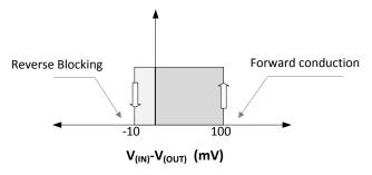
Figure 75. Active ORing Thresholds
