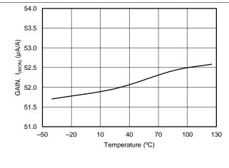
Figure 23. GAIN<sub>(IMON)</sub> vs Temperature
