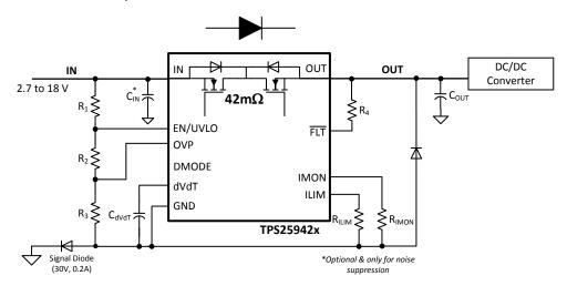
Figure 86. Reverse Polarity Protection Implementation
