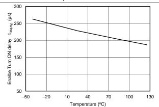
Figure 8. Enable Turnon Delay vs Temperature
