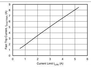
Figure 21. Fast Trip Threshold vs Current Limit
