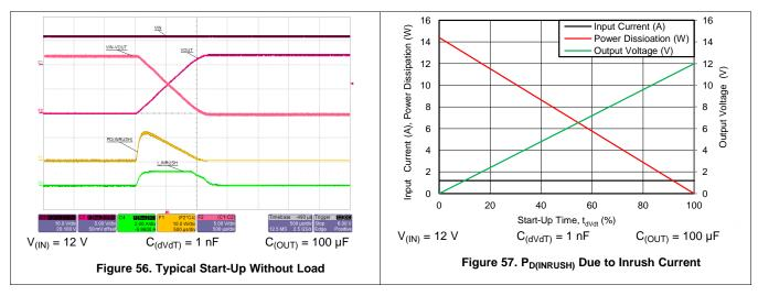
For the TPS25944, TPS25944 device, the inrush current is determined as shown in Equation 16.
