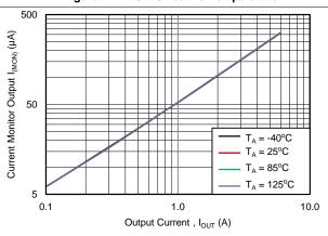
Figure 24. Current Monitor Output vs Output Current
