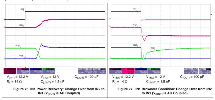
When bus voltages (IN1 and IN2) are matched, device in each rail sees a forward voltage drop and is ON delivering the load current. During this period, current is shared between the rails in the ratio of differential voltage drop across each device.
