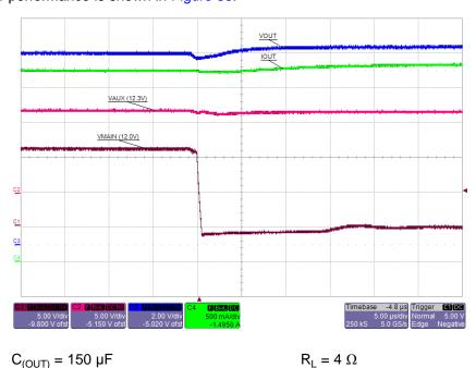
Figure 85. Brownout Condition: Diode Mode for Multiplexing
