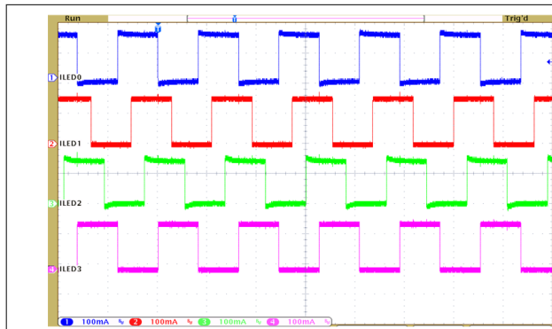
Figure 8-3. LED String Currents Showing Phase Shift PWM Operation
