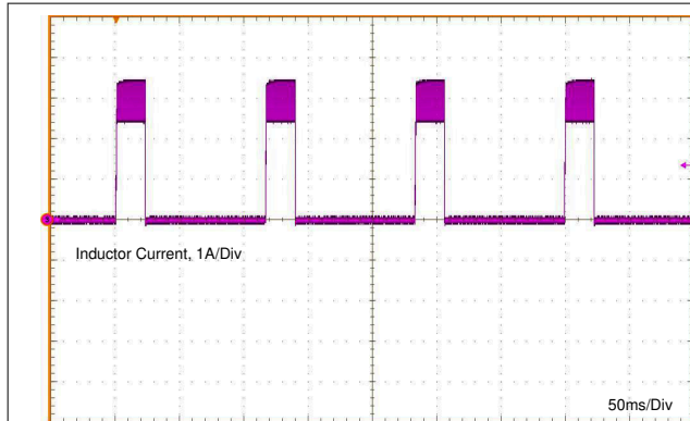
Figure 8-5. Inductor Current Burst in Short-Circuit Mode
