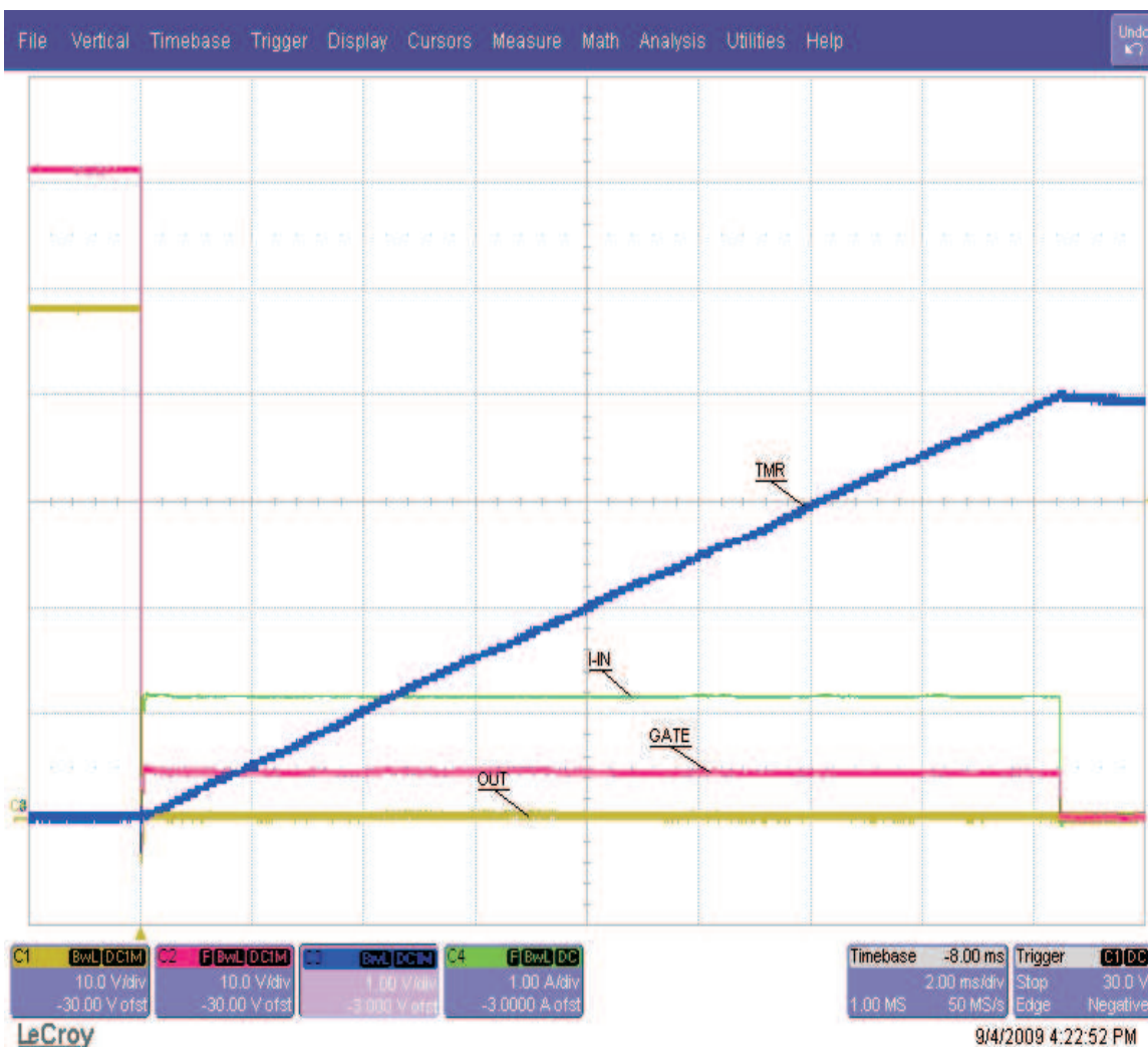
Figure 14. Current Limit Overview
