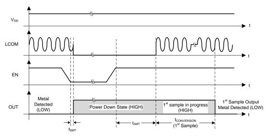
Figure 2. Shutdown and Resume Active Mode Timing Diagram
