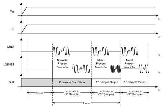
Figure 1. Start-up and Delay Time Diagram
