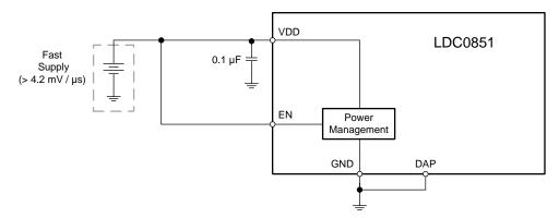
图 32. Supply Connections for Fast Ramp Rate
