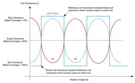
图 27. Angular Position vs Coil Inductance
