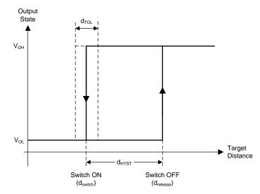
图 23. Switching Distance Hysteresis and Threshold Tolerance
