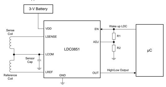
图 30. Application Schematic Showing Low Power Operation
