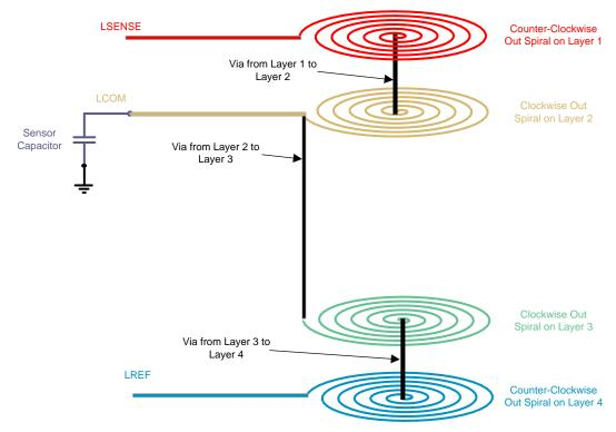
图 35. Stacked Coil Recommended Connections and Direction
