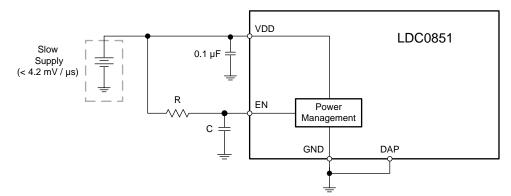
图 33. Supply Connections for Slow Ramp Rate
