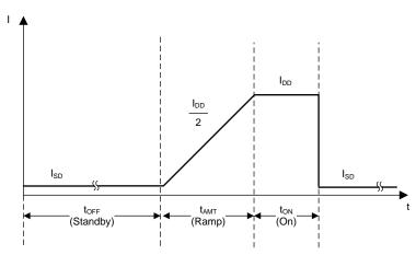
图 31. LDC0851 Supply Current vs. Time During Duty Cycle Operation
