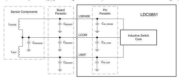
图 25. Sensor Components, Board Parasitics, and Package Parasitics Diagram
