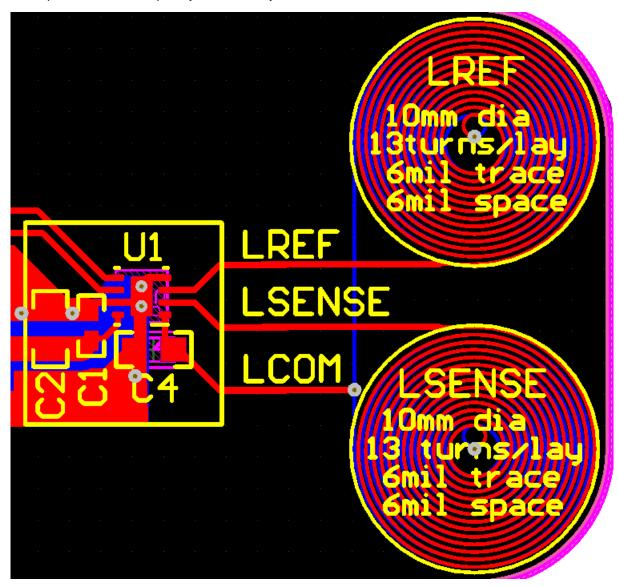
图 34. Side by Side Coil Layout Example
