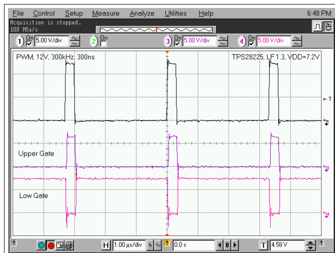
Figure 23. 12-V PWM Pulse at V_{DD} = 7.2\text{ V}
