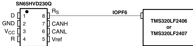
Figure 29. R_S (Pin 8) Connection to a TMS320LF2406/07 for High-Speed or Standby Mode Operation
