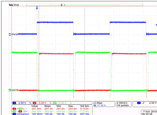
Figure 9-5. Bench Test Waveform for PWM and OUTA/B
