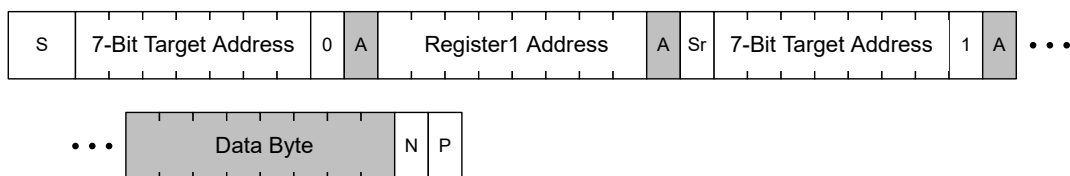
Figure 7-15. I 2 C Write Data Format
