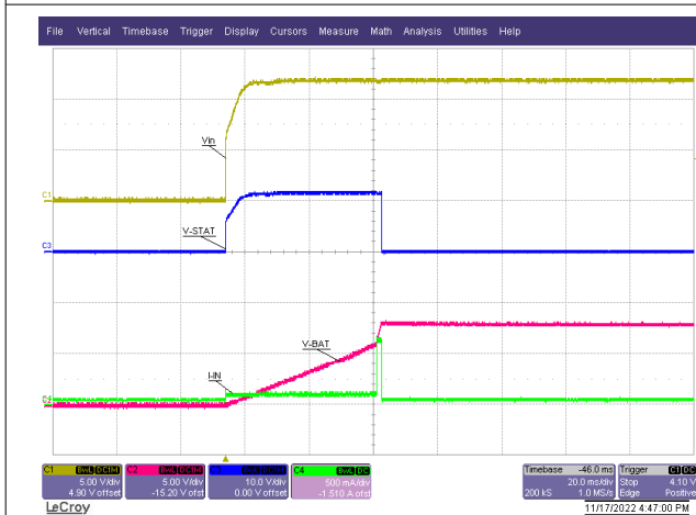
Figure 10-17. Power On - No Battery
