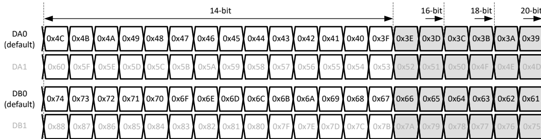
Figure 8-46. 1-wire output bit mapping
