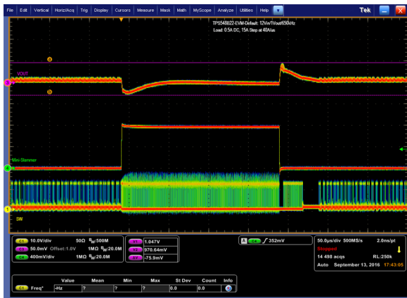
Figure 22. Output Voltage Regulation vs Output Current
