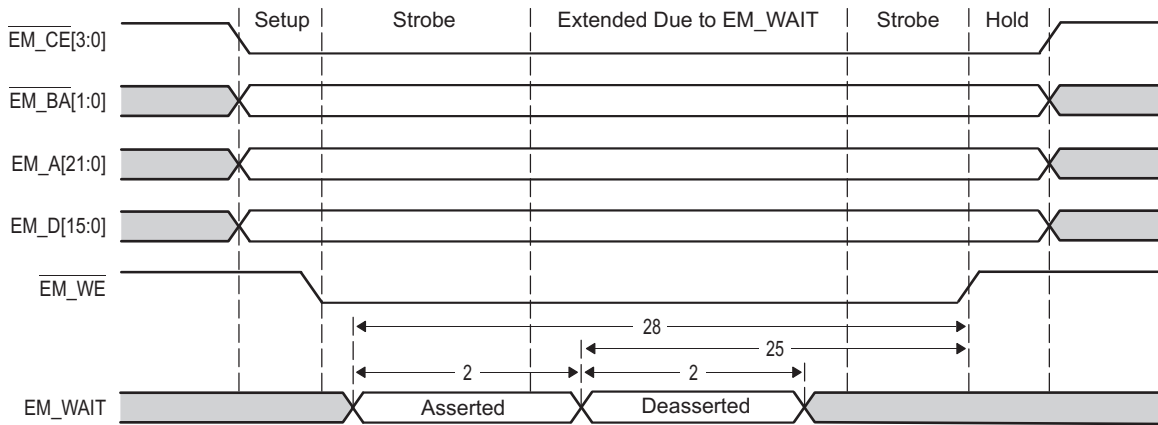
Figure 5-23. EMIF16 EM_WAIT Write Timing Diagram
