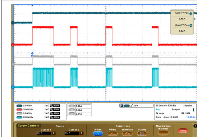
Figure 8-9. ITRIP Across TOFF and Load Current
