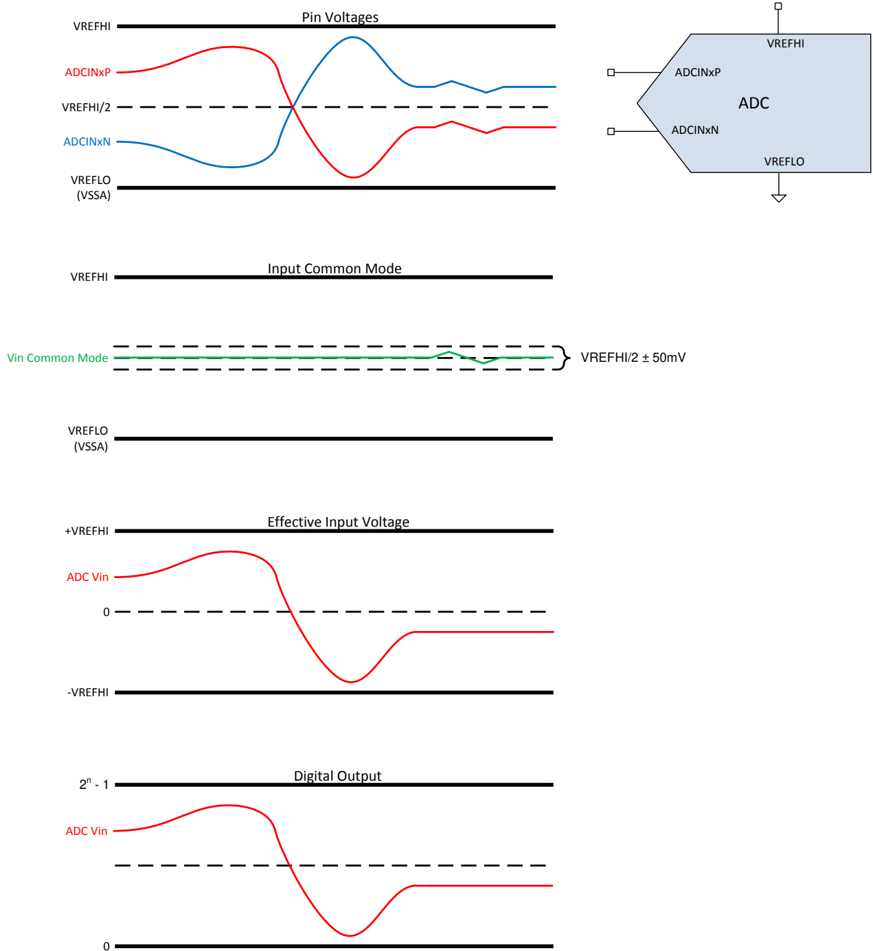
Figure 8-31. Differential Signaling Mode
