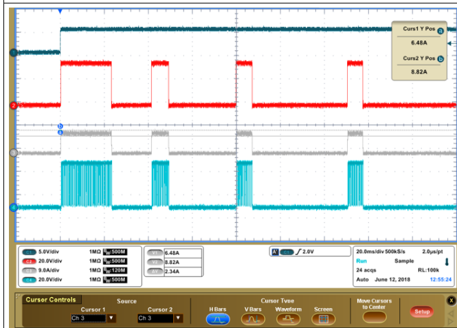
Figure 42. Overcurrent (OCP) Detection
