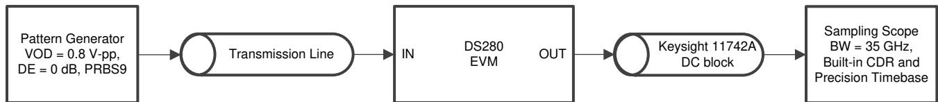
Figure 18. 5 in input Channel and Minimal Output Channel Test Setup
