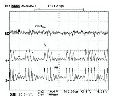
Figure 50. Operation in Pulse-Skip Mode
