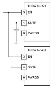
Figure 44. Schematic for Ratiometric Start-Up Using Coupled SS/TR Pins
