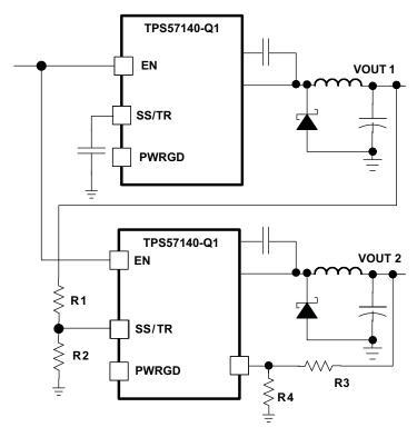
Figure 46. Schematic for Ratiometric and Simultaneous Start-Up Sequence
