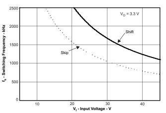
Figure 33. Maximum Switching Frequency vs Input Voltage
