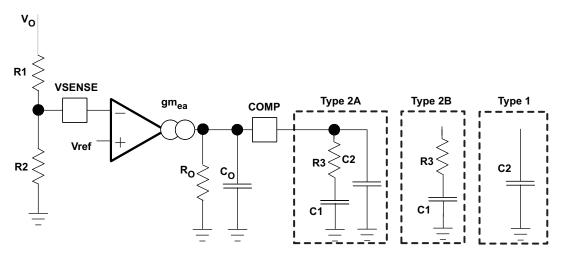
Figure 40. Types of Frequency Compensation
