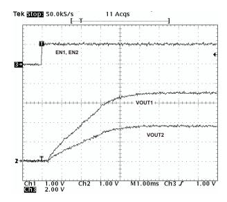
Figure 45. Ratiometric Start-Up Using Coupled SS/TR Pins
