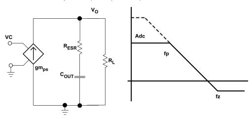
Figure 39. Simple Small-Signal Model and Frequency Response for Peak-Current-Mode Control
