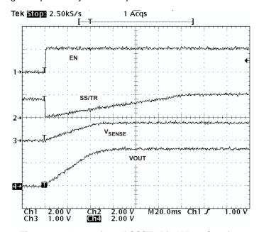
Figure 30. Operation of SS/TR Pin When Starting
