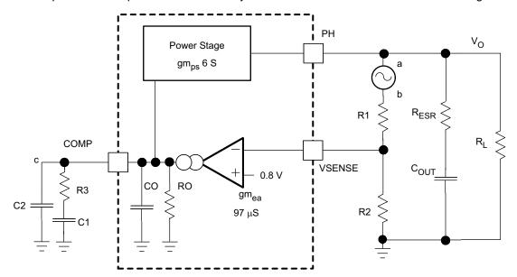
Figure 38. Small-Signal Model for Loop Response
