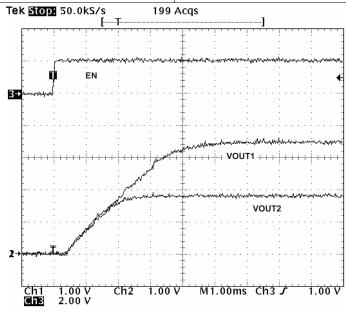
Figure 49. Simultaneous Start-Up With Tracking Resistor
