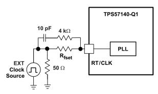
Figure 34. Synchronizing to a System Clock
