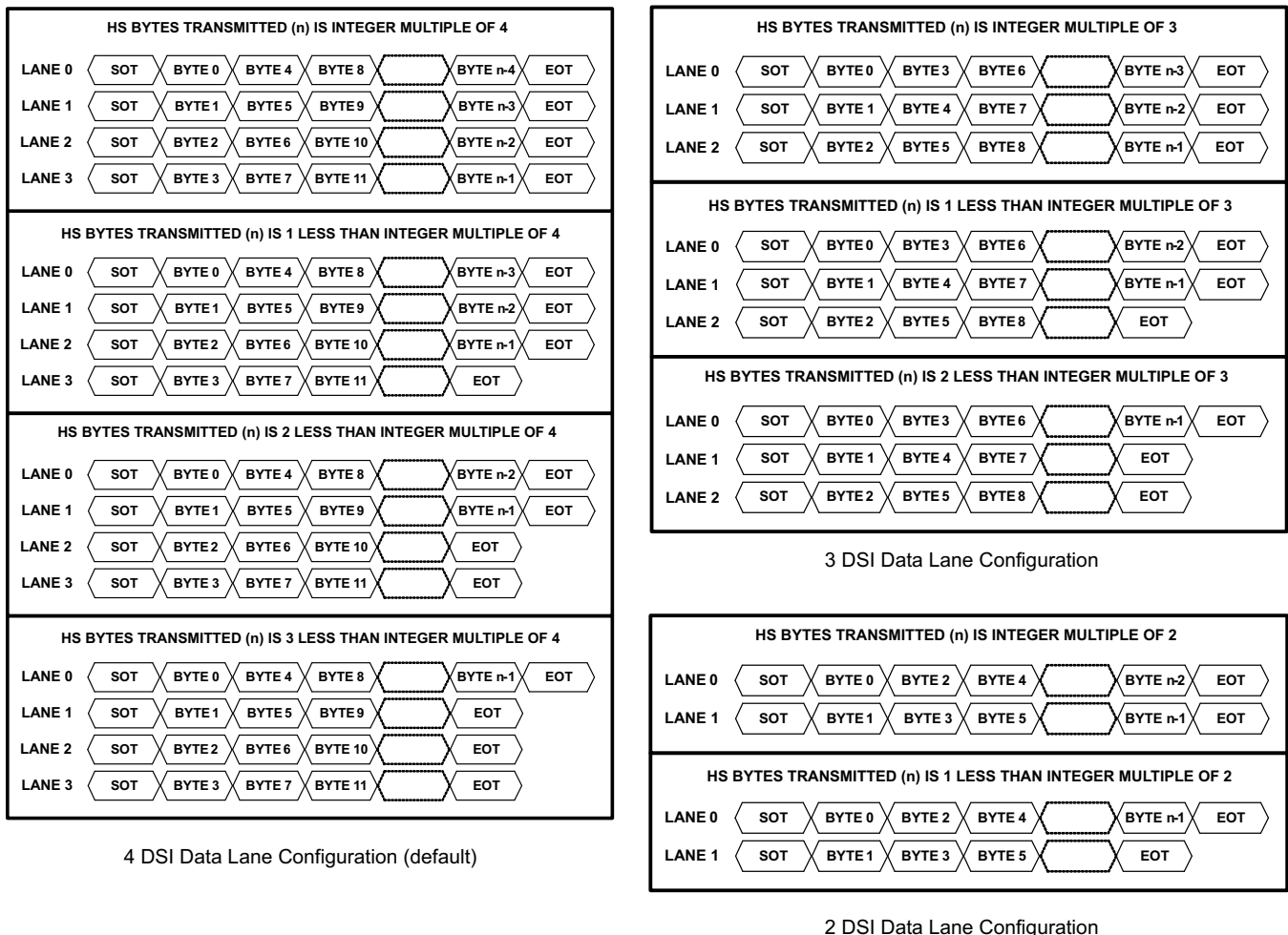
Figure 13. SN65DSI83-Q1 DSI Lane Merging Illustration
