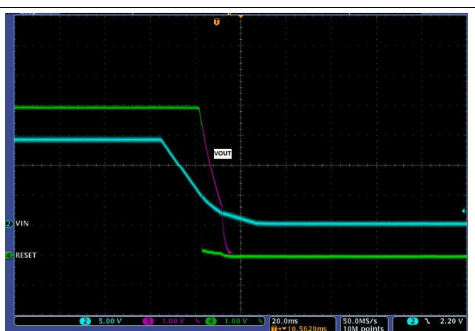
Figure 24. TPS7B6750-Q1 Power-Down Waveform
