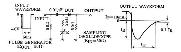
Fig.1 Reverse recovery time (t<sub>rr</sub>) test circuit
