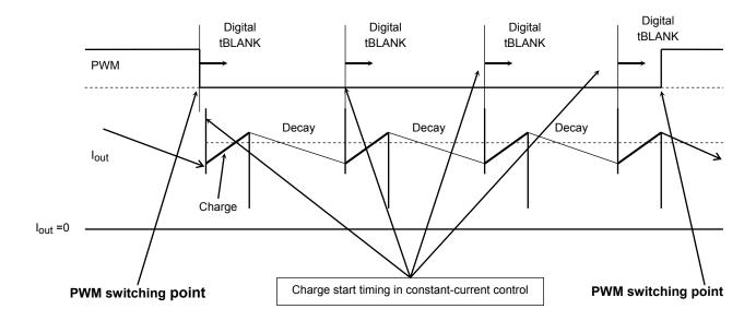
The digital tBLANK time is inserted immediately after the switching timing of externally applied PWM signals, PHASE\_X (such as the switching timing between short brake and charging), and also when the charging in constant-current chopper drive is started.
