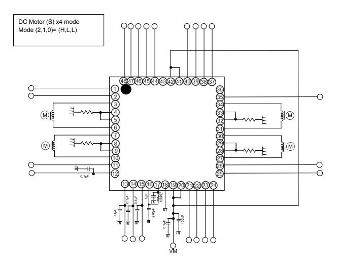
Note: It is recommended that a bypass capacitor is added if necessary. The GND wiring must become one-point-earth as much as possible.
