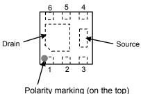
Polarity marking (on the top) \*Electrodes : on the bottom
