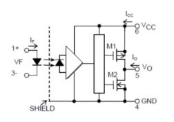
A ceramic capacitor (0.1  $\mu$ F) should be connected from pin 6 (VCC) to pin 4 (GND) to stabilize the operation of the high gain linear amplifier. Failure to provide the bypass may impair the switching property. The total lead length between capacitor and coupler should not exceed 1 cm.
