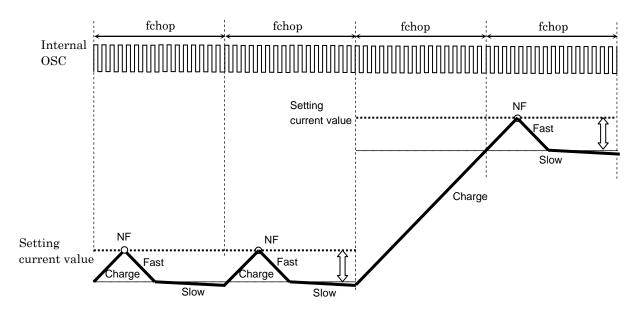
When the Charge period is longer than fchop cycle, the Charge period will be extended until the motor current reaches the NF threshold. Once the current reaches the next current step, then the sequence will go on to ADMD control.
