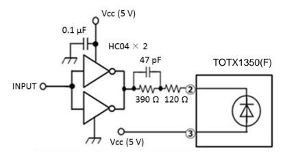
Replace 47 pF of capacitor with 82 pF if need a smaller jitter.
