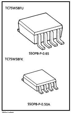
Weight SSOP8-P-0.65: 0.021g (typ.) SSOP8-P-0.50A: 0.01g (typ.)
