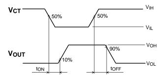
Figure 1 t<sub>r</sub>, t<sub>f</sub>, t<sub>ON</sub>, t<sub>OFF</sub> Waveforms
