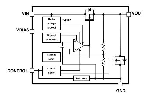
\* Under voltage lockout is applied TCR5BMxxA products.
