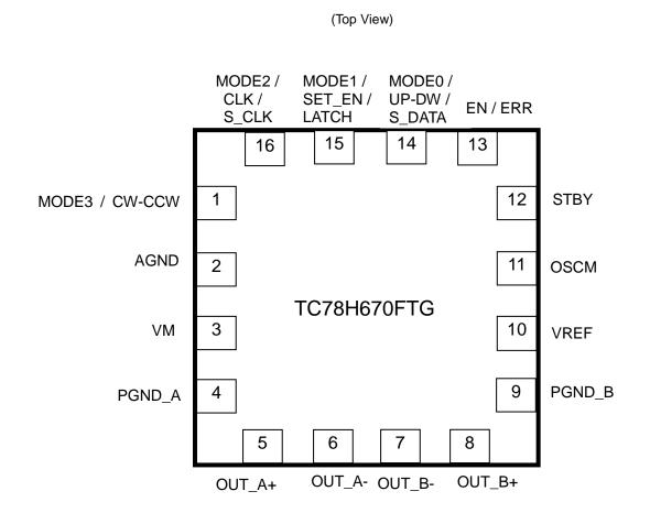
Note: Please solder the corner pads and the rear thermal pad of the QFN package, to the GND pattern of the PCB.
