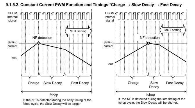
The Charge period (the time until the motor current reaches the set current value) is determined by the operating status. Therefore the NF detection timing (the motor current reaches the set current value) with the chopping cycle (fchop) may change. If NF is detected in the early period of the fchop cycle, the Slow Decay will be longer. If NF is detected in the late period of the fchop cycle, the Slow Decay will be shorter, as shown above.
