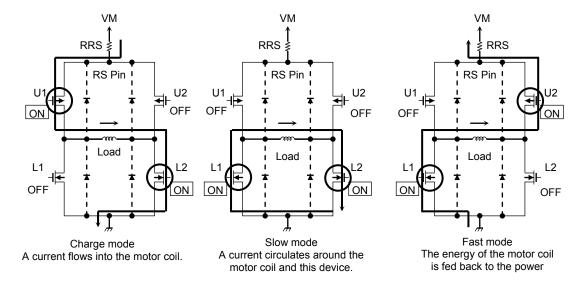
**Output transistor operational function**
