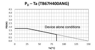
This value is dependent on a substrate pattern and mounting conditions. Moreover, when ambient temperature is high, permissible power consumption becomes small.
