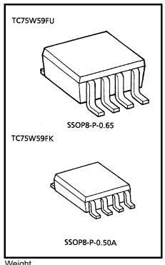
Weight SSOP8-P-0.65: 0.021g (typ.) SSOP8-P-0.50A: 0.01g (typ.)
