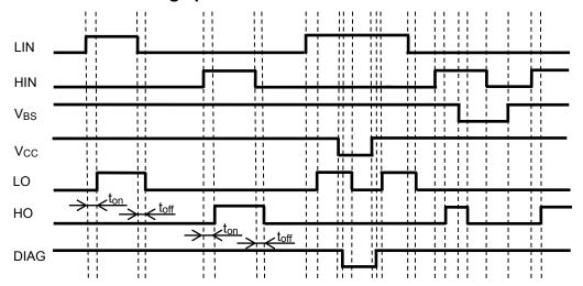
Note: The above timing chart is considering the delay time
