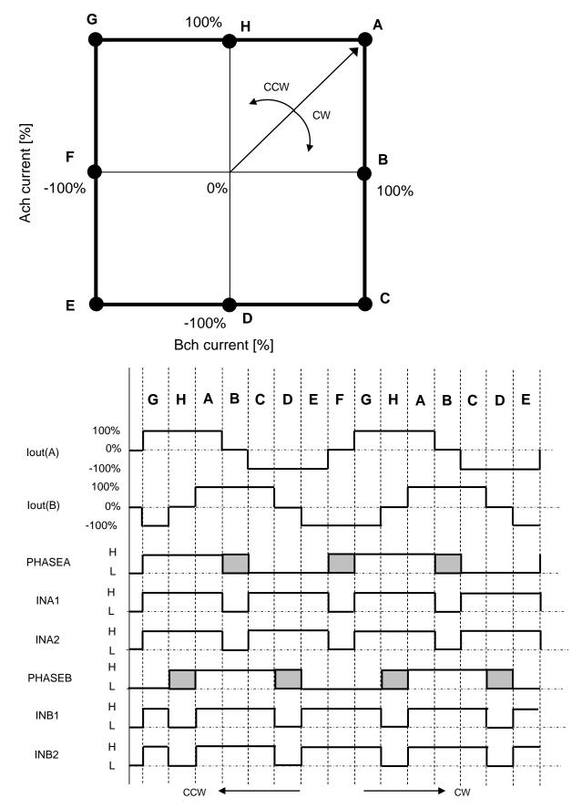
Timing charts may be simplified for explanatory purpose. Please set INA1, INA2, INB1, and INB2 to Low until VM power supply reaches the proper operating range.
