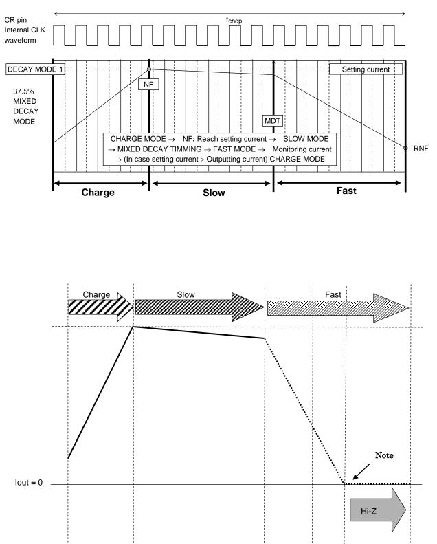
Note: When the motor current reaches the 0A level, the output transistor will turn to "Hi-Z" status.
