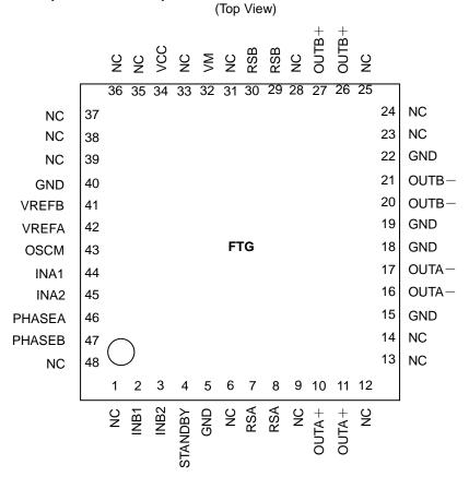
Please mount the four corner pins of the QFN package and the exposed pad to the GND area of the PCB.
