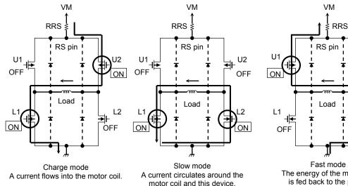
The energy of the motor coil is fed back to the power
