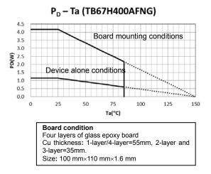
This value is dependent on a substrate pattern and mounting conditions. Moreover, when ambient temperature is high, permissible power consumption becomes small.
