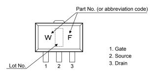
Caution: This device is sensitive to electrostatic discharge.
