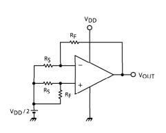
• SVRR  $V_{DD} = 1.8V : V_{DD} = V_{DD}1, V_{OUT} = V_{OUT}1$   $V_{DD} = 7.0V : V_{DD} = V_{DD}2, V_{OUT} = V_{OUT}2$  $SVRR = 20 \log \left( \left| \frac{V_{OUT}1 - V_{OUT}2}{V_{DD}1 - V_{DD}2} \right| \times \frac{R_S}{R_F + R_S} \right)$
