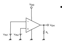
$V_{OH}$  $V_{IN1} = \frac{V_{DD}}{2} - 0.05V$  $V_{IN2} = \frac{V_{DD}}{2} + 0.05V$
