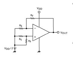
• SVRR  $V_{DD} = 1.5V$  :  $V_{DD} = V_{DD}1$ ,  $V_{OUT} = V_{OUT}1$   $V_{DD} = 7.0V$  :  $V_{DD} = V_{DD}2$ ,  $V_{OUT} = V_{OUT}2$  $SVRR = 20log\left(\left|\frac{V_{OUT}1 - V_{OUT}2}{V_{DD}1 - V_{DD}2}\right| \times \frac{R_S}{R_F + R_S}\right)$
