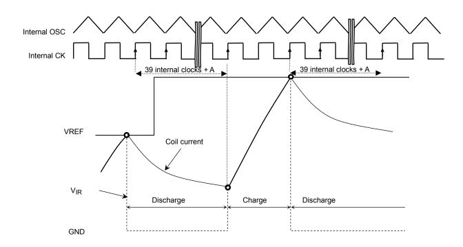
Due to the peak current detection technique, the average current value of the constant-current operation shall be smaller than the predetermined value. Because this depends on characteristics of used motor coils, precise identification of the used motor coils must be performed when determining the current value.
