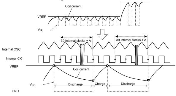
(4) Operation on change of predetermined current value (when in Discharge mode)
