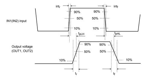
Note: When the signal is input to IN1 (IN2) pin, we recommend that intr, intf are provided more than 10ns in order to avoid malfunction in the input switching noise. For example, please connect the capacitor between IN1 (IN2) pin and GND.
