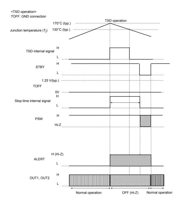
Note: The TSD circuit is activated if the absolute maximum junction temperature rating  $(T_j)$  of 150°C is violated. Note that the circuit is provided as an auxiliary only and does not necessarily provide the IC with a perfect protection from any kind of damages.
