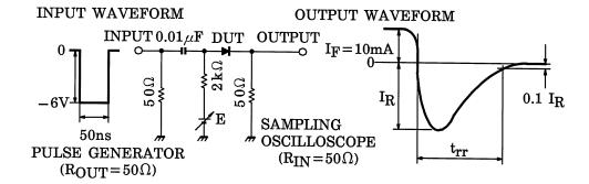
Fig.1 Reverse Recovery Time (t<sub>rr</sub>) Test Circuit
