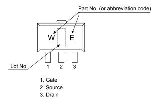
**Caution:** This device is sensitive to electrostatic discharge.
