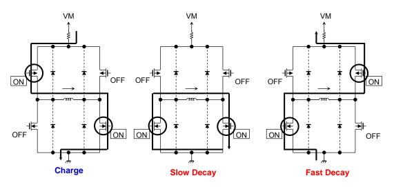
\* The TB67H401FTG has a 400ns (design target, fixed value) dead time to avoid any flow-through current during switching.
