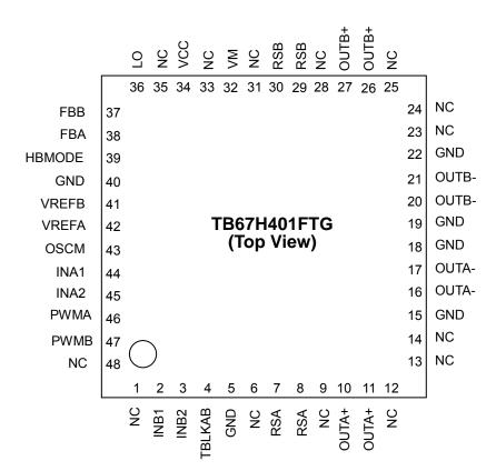
Note: Please solder the corner pad and the bottom thermal pad of the QFN package, to the GND pattern of the PCB. Note: Pin names in the above figure are in the state when HBMODE pin is low level.
