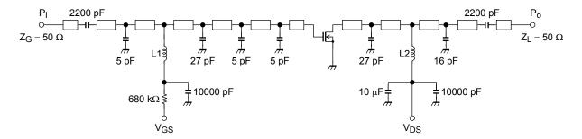
L1:  $\phi$ 0.6 mm enamel wire, 5.8ID, 8T L2:  $\phi$ 0.6 mm enamel wire, 5.8ID, 8T
