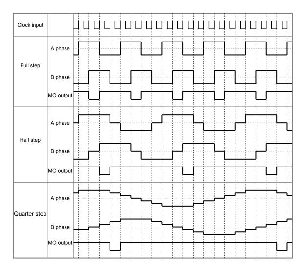
MO output shown in the timing chart is when the MO pin is pulled up.
