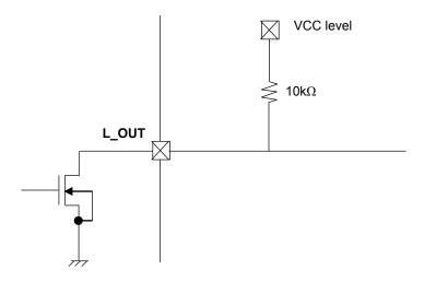
The LO is an open-drain output pin. LO pin needs to be pulled up to 3.3V/5.0V level for proper function. During regular operation, the LO pin level will stay High(VCC level). When error detection (TSD, ISD) is applied, the LO pin will show Low (GND) level.
