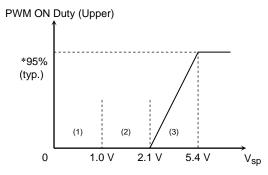
\*: The maximum ON duty is  $T_{on} = 95\%$  (typ.) when  $V_{SP} = 5.4 \text{ V}$  (typ.). Example: If  $f_{OSC} = 5$  MHz, then ON time = 48  $\mu s$  (typ.) ( $f_C = 19.8$  kHz)
