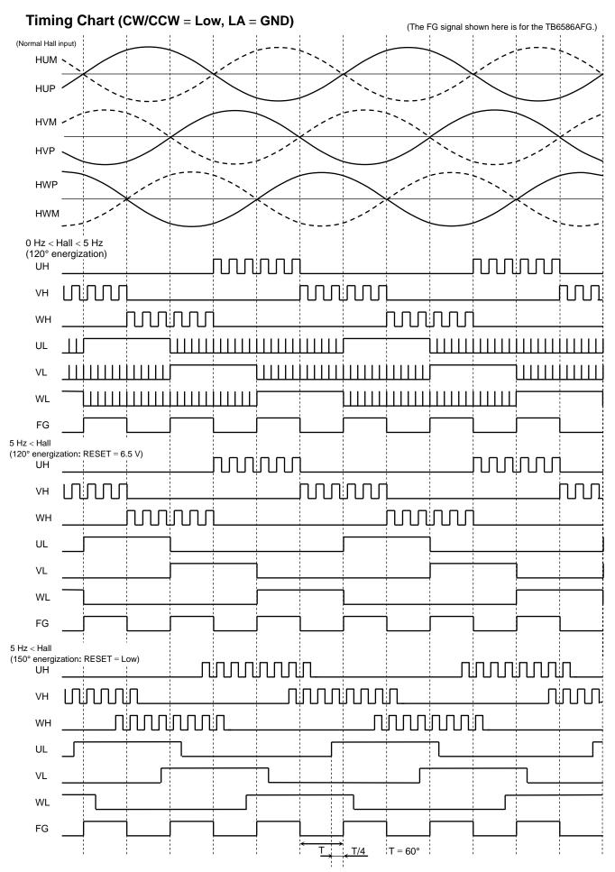
\*: When the Hall signal is 5 Hz or higher, the lead angle function operates in accordance with the LA pin. signal.
