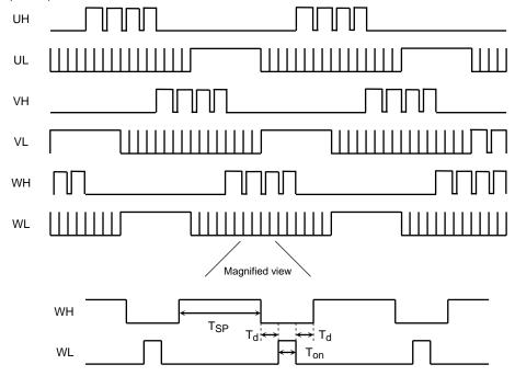
$T_{SP}$ : Variable depending on the  $V_{SP}$  (the figure above being applicable when  $V_{SP} = 5.4$  V (typ.));  $T_{ON} = 18/f_{OSC}$ ;  $T_{OSC} = 18/f_{OSC}$
