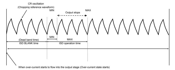
The over-current detection circuit has a dead band time to prevent erroneous detection of  $I_{RR}$  or spike current at switching. The dead band time being synchronized with the frequency of the OSC for setting chopping frequency is expressed as follows.
