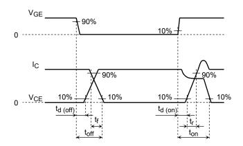
Note 2: Switching loss measurement waveforms
