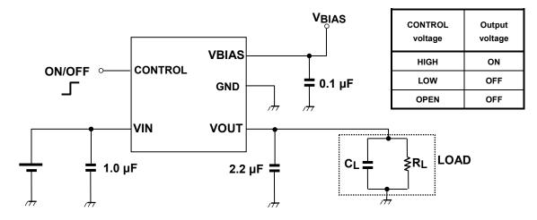
The figure above shows the Example of configuration for using a Low dropout regulator. Insert a capacitor at VIN, VOUT and VBIAS pins for stable input/output operation. (Ceramic capacitors can be used).
