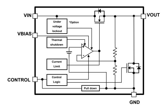
\* Under voltage lockout is applied TCR8BMxxA products.
