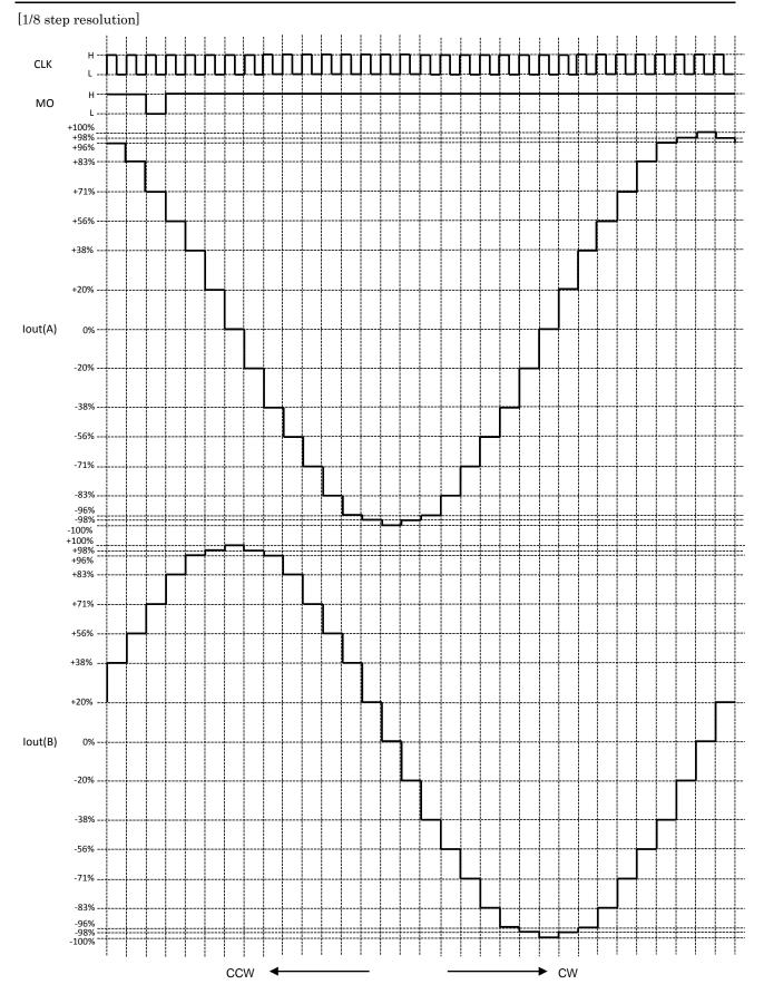
MO output shown in the timing chart is when the MO pin is pulled up.
