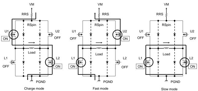
Charge mode A current flows into the motor coil.
