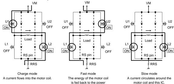
**Operation Function of Output Transistor**
